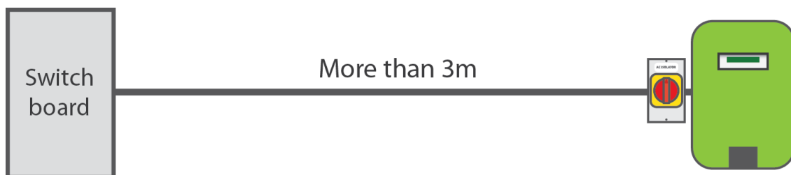
Figure 23: a.c. switch-disconnector is required when distance is greater than 3m or the switchboard is not visible from the inverter
